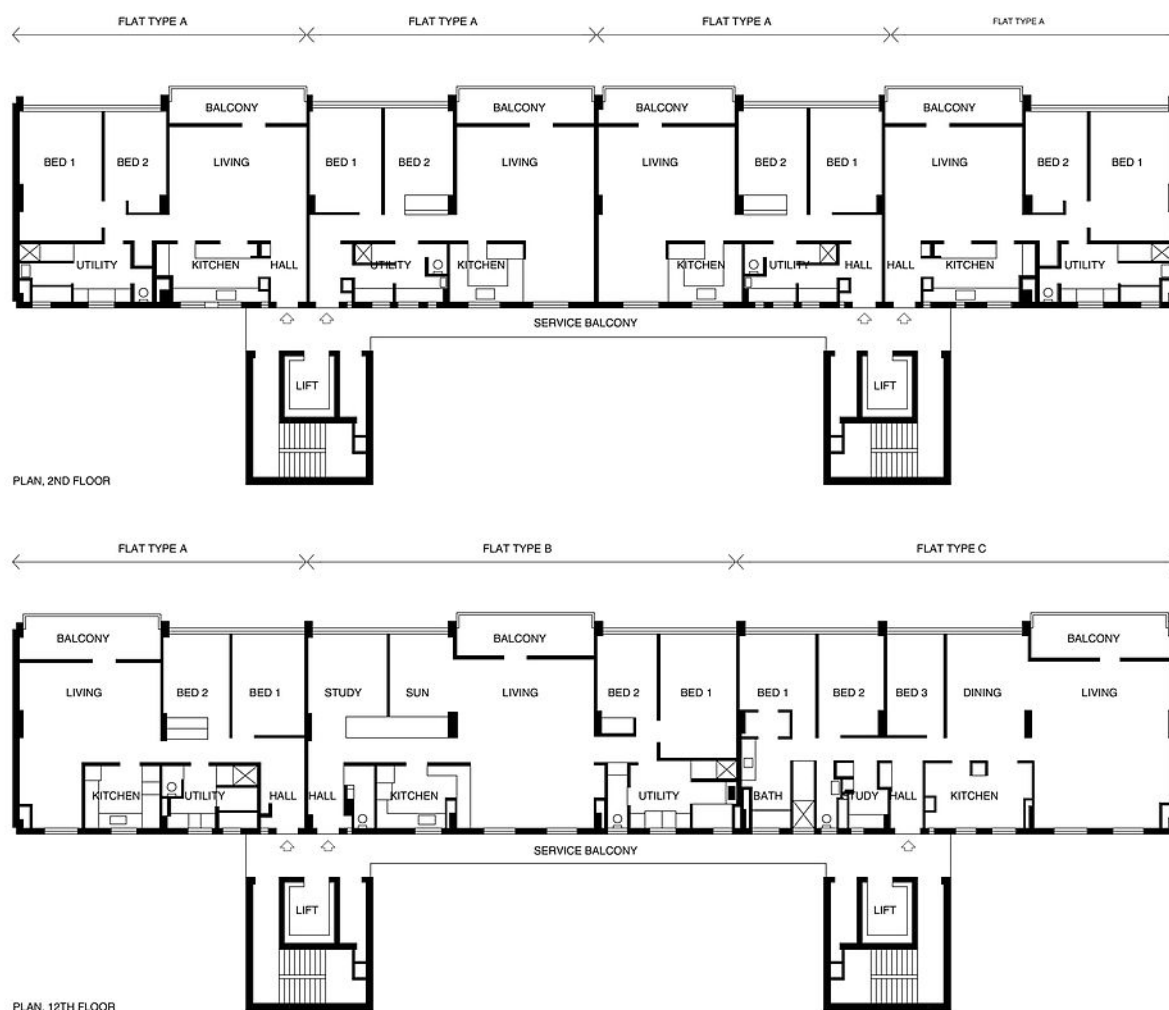
Figure 5. Plan of internal layout on the second and 12th floors, showing flat types A-C. (Source: Ben Brendan 2013 via Wikimedia Commons)
